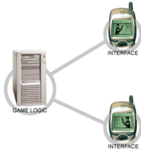
Figure 2: WAP phones are dumb user interfaces, all game logic resides on the server
